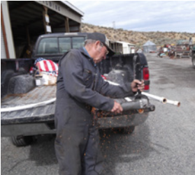
Kent Blomgren cutting off end of flag poles to make them fit into the bracket
