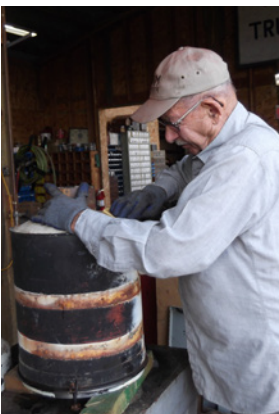
Mike Stump sanding the water truck air cleaner
