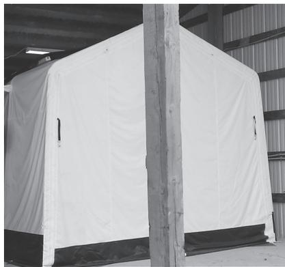
**The new paint booth, which is ventilated for safety will be used to paint restored equipment.**
