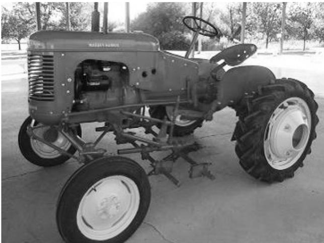
The biggest selling tractor produced by Massey-Harris before the merger with Ferguson, was the little one-furrow Pony. The tractor went into production at the Woodstock factory in Canada in 1947 and was also produced in France at the Marquette plant from 1951. When the last of the Pony tractors was built in 1961, the production total had reached more than 121,000.
