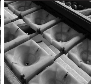
The sizing cups in the apple packing line are being replaced
